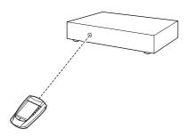
You can select to operate devices using radio frequency (RF) signals instead of IR signals. RF signals have an operating distance of approximately 20 meters (66 feet) in house and , unlike IR signals, is able to go through obstacles like furniture or walls. The RF signals sent out by the remote controller are picked up by the RF Receiver. The RF Receiver translates the RF signals in IR signals and sends the IR signals to the appropriate device.
